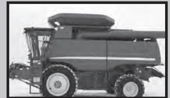
The AMX27359 Tip-Up adds approximately 60 bushel capacity.
