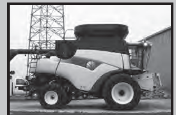
The AMX27370, AMX27372 and AMX27373 Tip-Up adds approximately 100 bushel capacity.
