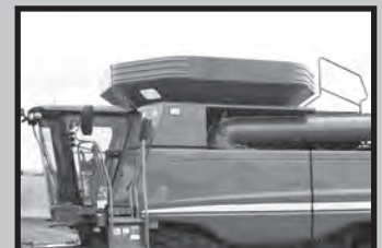
The AMX27360 Tip-Up adds approximately 120 bushel capacity.
