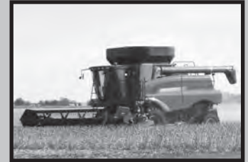
The AMX27371 Tip-Up adds approximately 100 bushel capacity.
