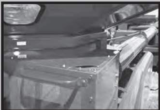
Corner Caps on all Case IH® Gen II extensions prevent leakage.
