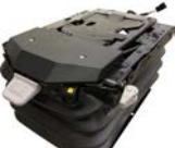
For Grammer Seat Assemblies | Suspension, Air<br>For 24 Volt Systems<br>• Grammer MSG95G air suspension<br>• Self-contained 24-volt compressor<br>• Frame width of 11.75"<br>• Side controls<br>• Fore/aft isolator<br>• Air suspension with suspension travel of 4"<br>• Suspension stroke up to 7"<br>• Adjustable to suit driver's weight from 110 to 285 lbs<br>• Weight indicator<br>• Shock absorber | AM1319709   | \$ 583.00    |
